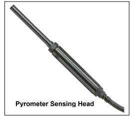
The robust sensing head employs a DC operated detector with direct digitalization of the temperature signal. This extremely insensitive to interference signal is transferred through a hermetically sealed flexible braided steel hose to the main electronic processor, which can be installed remotely in a less severe environment. The hose can be 30 m long and provides a conduit for air purging and cooling of the sensing head also.
