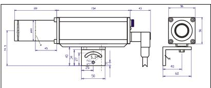
Depending on type, length of lens tube is either 45 mm or 89 mm.
