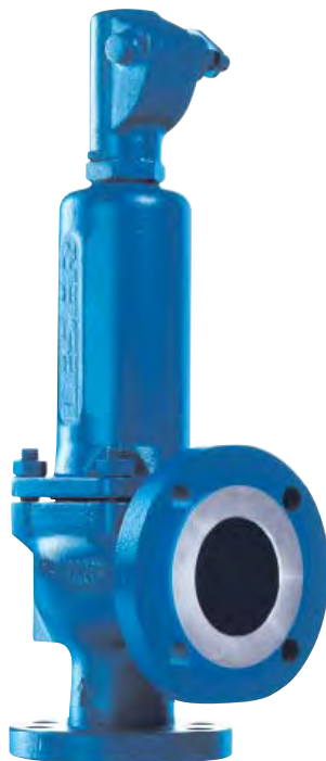
Type 442 Full nozzle Plain lever H3 Bonnet open Conventional design
