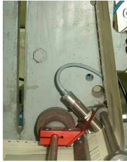
Fig. 2: Glue line detection with flush mountable sensors
