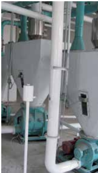
Fig. 6: Level control or road salt
