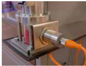
Fig. 3 to 5: Level control of granules, powder or bulk material
