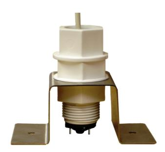
The sensor has been designed to detect the presents of oil or any non-conductive liquid including fuel oil, diesel etc. and energise an internal relay to provide a signal to existing alarm systems, Building Management Systems or SMS messaging systems.
