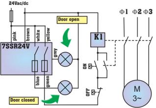
Note: the yellow/green line of the 7SSR24V is closed in case of lack of power supply.
