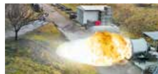
Thermographic investigation of a dust explosion: conventional explosion venting with an explosion vent.
