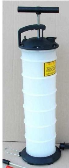
**OIL EXTRACTOR:** Hand vacuum pump used for extracting or changing engine oils in motor vehicles, motor bikes, marine engines and stationary engines.
