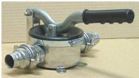
**BARADELLO MINI PUMP:** Hand pump with body and couplings made of stainless steel, single diaphragm, self-priming and single acting. MARINA version is for boats.
