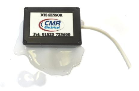
The sensor has been designed to detect the presence water in drip trays and energise an internal relay to provide a volt free contact signal to existing alarm systems, Building Management Systems or SMS messaging systems.
